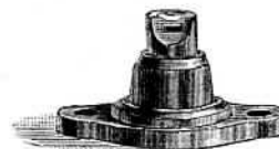
Small Stand and Punch for Fixing Eyelet Hooks,
